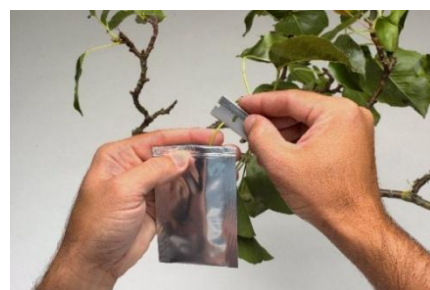
Figure 24 - Stem Water Potential with bagged leaves, PMS Instrument Company
