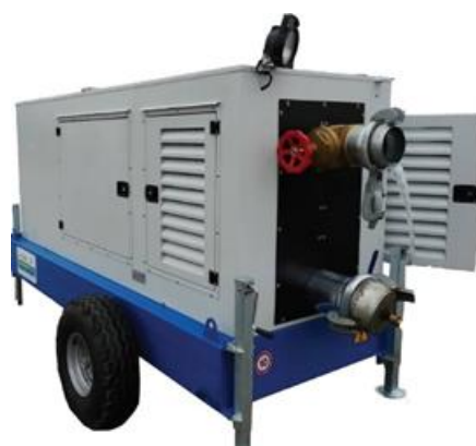
Figure 33 - Mobile pump system
