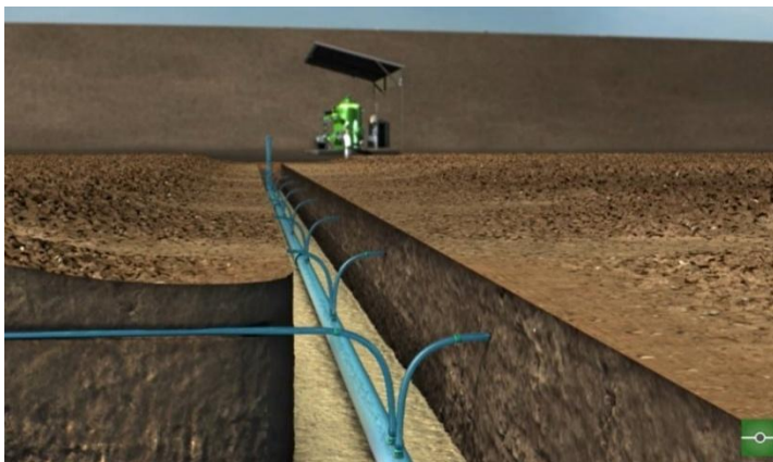
Figure 18 - Subsurface Drip, Rivulis
